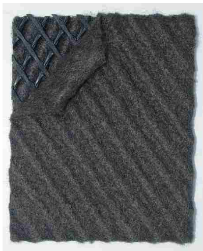
Figure A-2 Geocomposite
